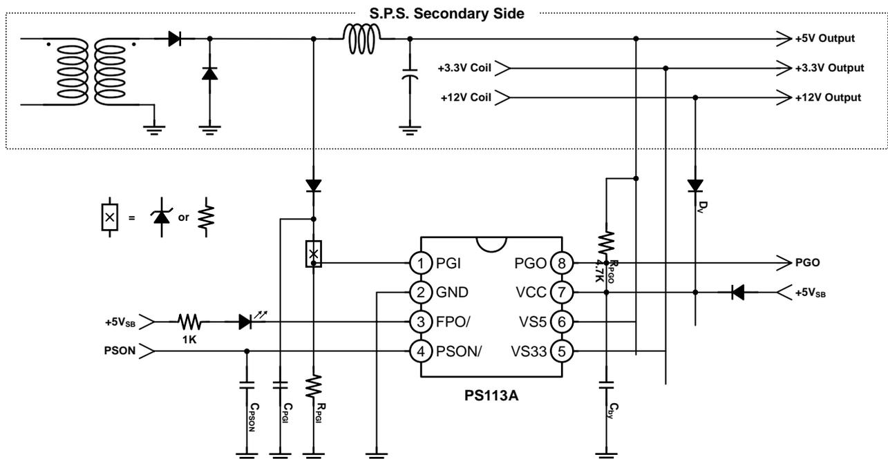
Note1: Zener diode or resistor or both of them can be used in component X.
